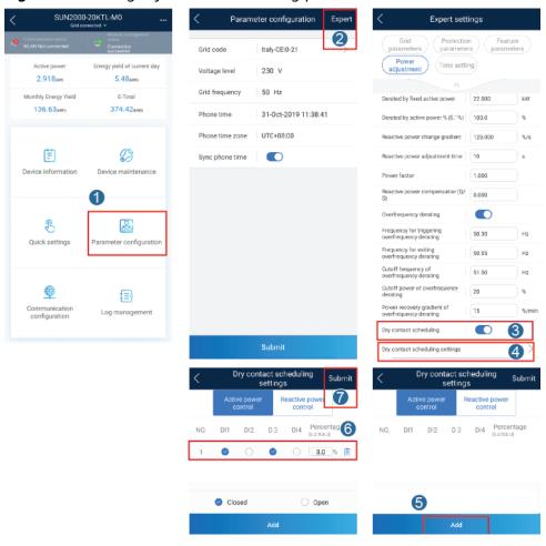
Figure B-1 Setting dry contact scheduling parameters
