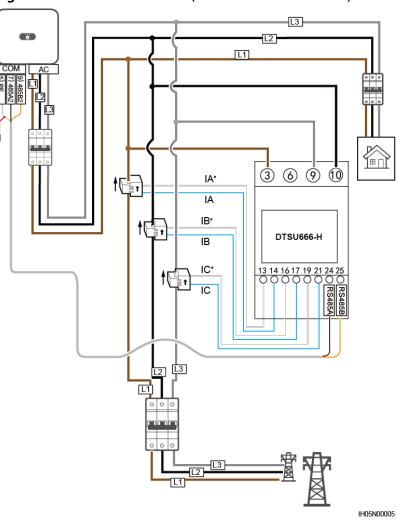
Figure 5-24 Cable connection (Three Phase Three Wire)
