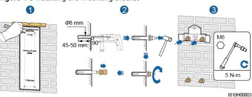
Figure 4-9 Installing the Mounting Bracket
