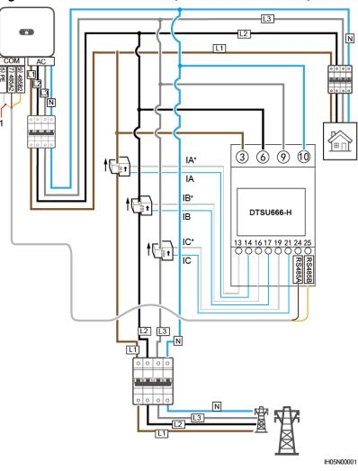
Figure 5-25 Cable connection (Three Phase Four Wire)
