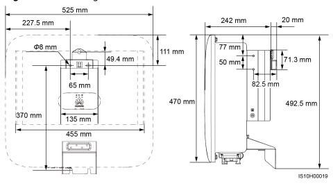
Figure 4-7 Mounting bracket dimensions
