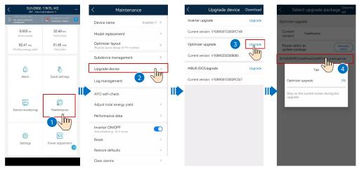
If the optimizer upgrade is successful, the alarm "2065-7 Upgrade Failed or Version Mismatch" will be automatically cleared, and the inverter will be reconnected to the power grid.
