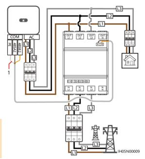
(1) Shield layer of the signal cable
