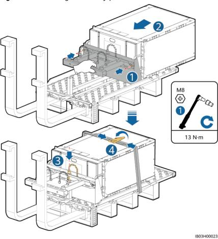
Figure 7-19 Securing the battery pack
