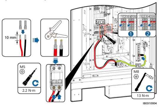
Figure 8-16 Connecting the cable
