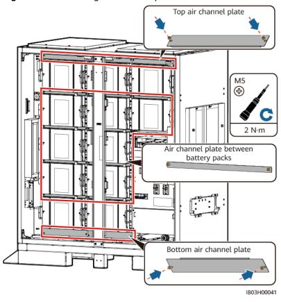
Figure 7-22 Installing air channel plates
