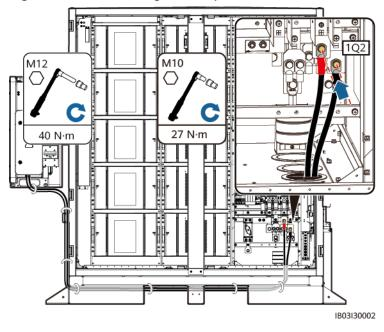
Figure 8-14 Connecting the DC power cable
