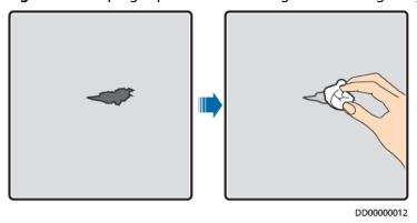
**Step 3** Paint zinc-rich primer on the damaged coat using a brush or paint spray gun.
