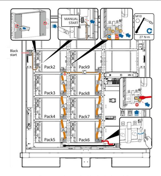
Figure 8-5 Installing copper bars and cables (97 kWh model)
