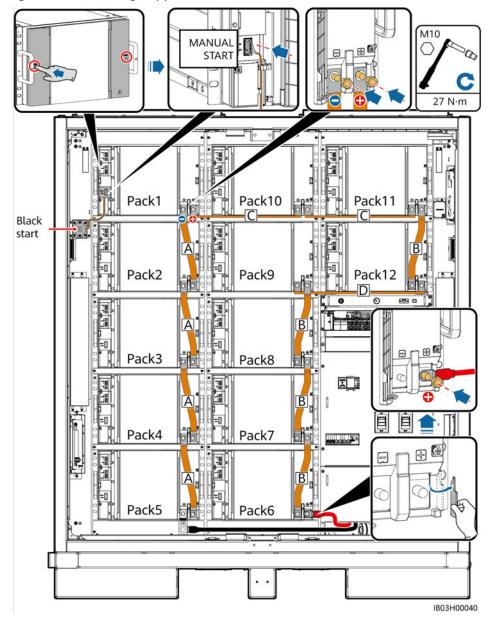
Figure 8-2 Installing copper bars and cables (200 kWh model)
