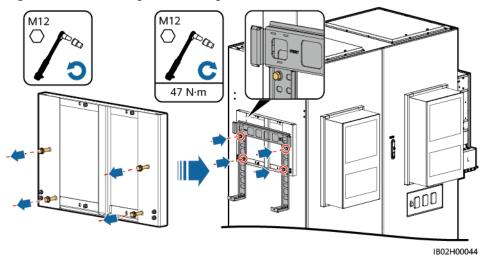
Figure 7-31 Installing a mounting bracket
