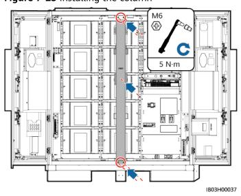
Figure 7-23 Installing the column
