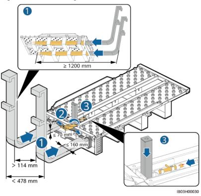
Figure 7-16 Assembling the installation kit
