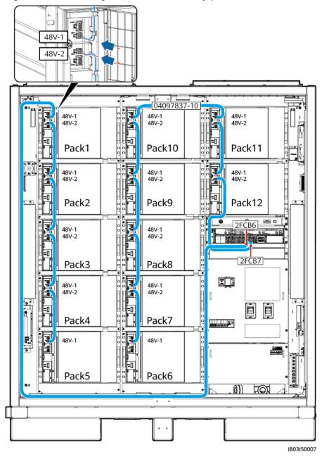
Figure 8-6 Connecting 48 V cables to battery packs
