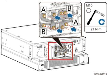
**Figure 7-26** Installing short-circuiting copper bars (97 kWh/129 kWh/161 kWh model)
