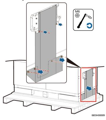
Figure 7-1 Removing the bottom baffle
