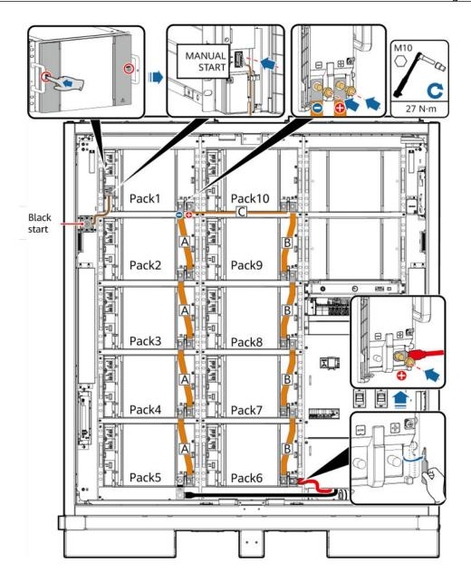
Figure 8-4 Installing copper bars and cables (129 kWh model)
