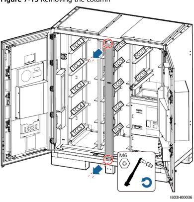
Figure 7-13 Removing the column
