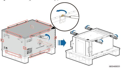
**Step 6** Install the operating handle on the battery pack, place the battery pack on the installation kit, and secure the battery pack.
