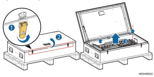
Figure 7-15 Taking out the installation kit
