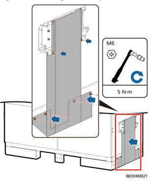
Figure 7-3 Installing the baffle plate
