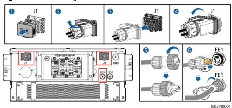
Figure 8-11 Connecting cables
