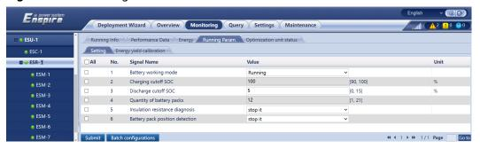
**Step 3** Choose **Monitoring** > **ESR** > **Running Param.** > **Setting** and set **Quantity of battery packs** to the actual quantity of installed battery packs.
