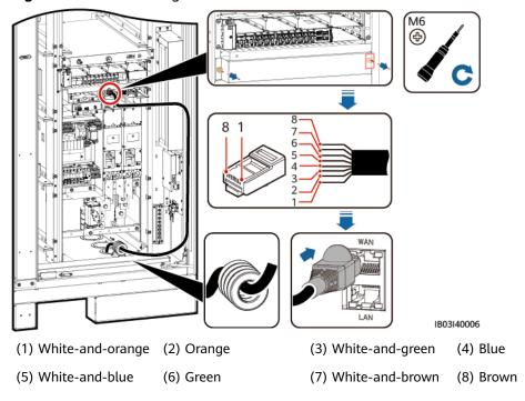
Figure 8-17 Connecting the FE communications cable
