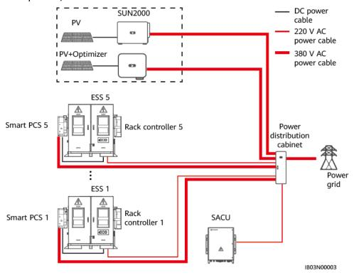
Table 2-22 1.0 MWh/500 kW standard solution configurations
