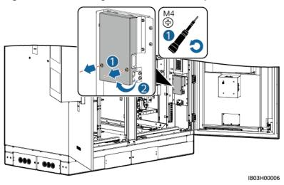
**Step 2** Remove the optical fiber cable fastener.
