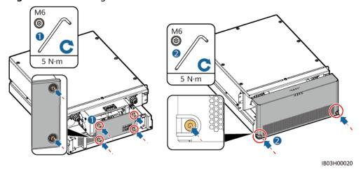
**Step 5** Install the protective covers delivered with the product, connect a ground cable to the protective cover on the left or right side, and bind the cable.
