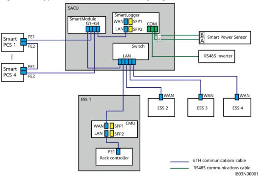
Figure 2-32 Typical communication networking diagram (FE)
