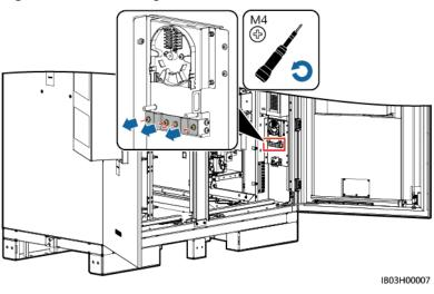
Figure 8-20 Removing the fastener
