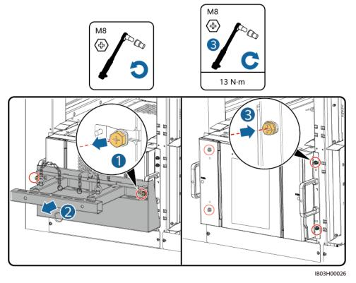
**Step 9** Install air channel plates between battery packs based on the label on the air channel plates. The air channel plates are delivered with the product.
