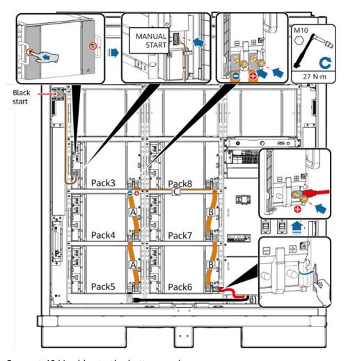
**Step 2** Connect 48 V cables to the battery packs.
