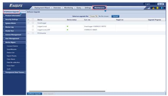
**Step 2** After the software upgrade is complete, the SmartLogger automatically restarts. Log in to the SmartLogger WebUI again 2 minutes later.
