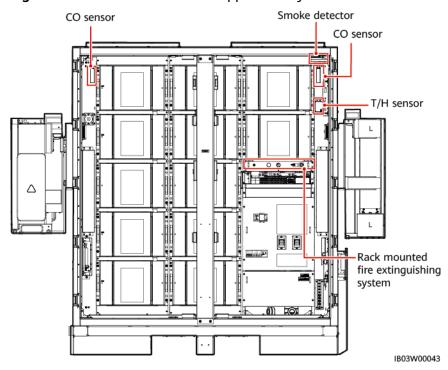
Figure 2-19 Position of the fire suppression system
