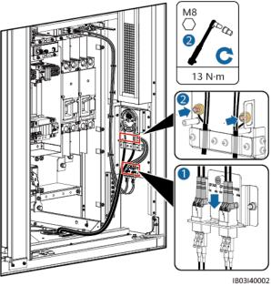
**Step 6** Check that the cables are connected correctly and securely. Then reinstall the optical fiber cable fastener and external mechanical parts.
