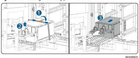
Figure 7-20 Installing the battery pack in the ESS
