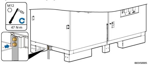
Figure 7-10 Connecting a ground flat steel sheet
