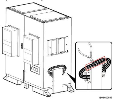
Figure 7-28 Removing bound cables
