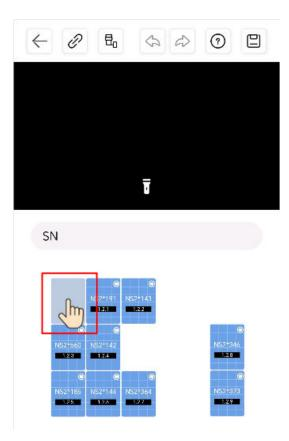
indicates the 1:1 scenario where one optimizer is bound to one PV module.
