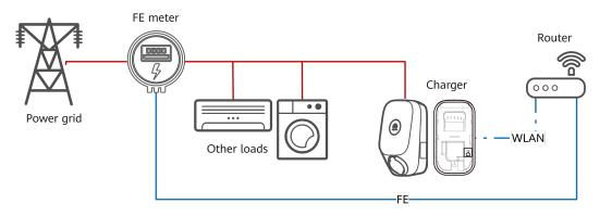
Figure 6-3 Charger connected to a router through WLAN
