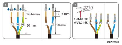
**Step 2** Connect the non-backup load output power cable.
