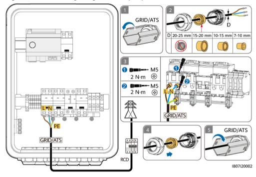
Figure 5-7 Connecting the grid AC output power cable
