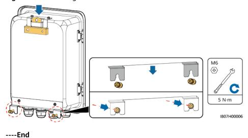
Figure 4-10 Installing the SmartGuard
