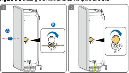
Figure 6-3 Closing the maintenance compartment door
