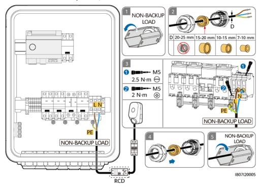
**Figure 5-14** Connecting the non-backup load output power cable (the component in the dashed box is optional)
