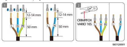
**Step 2** Connect the grid AC output power cable.
