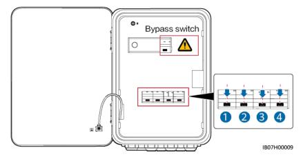
2. Remove the bypass switch latch, turn on the bypass switch, and then turn on switches **1** and **4** shown in the figure.
