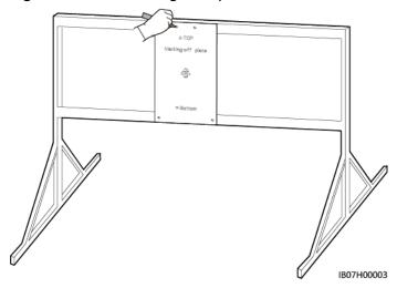
**Step 2** Drill holes using a hammer drill.
