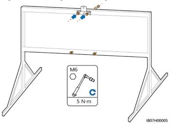
Figure 4-9 Securing the mounting bracket
