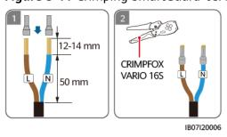
**Step 2** Connect the backup load output power cable.
